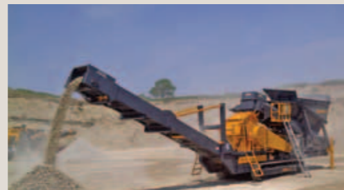
Crushed Material Exits Crusher and up Product Conveyor
