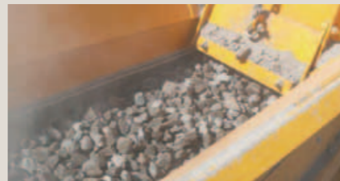
The Material to be Crushed is conveyed to the 623 Crushing Chamber
