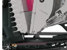
The large gap between crusher discharge and main conveyor belt, paired with wide main and side conveyors result in an optimized material flow.
