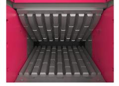
Deep 1.91m jaw chamber with single toggle design accommodates hard rock applications and large feed sizes. Also features closed side setting adjustment with hydraulic wedges.
