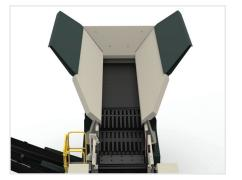
Double deck grizzly pre-screen featuring hydraulic fold and wedge lock hopper, and optional cassettes - punch plate or fingers.
